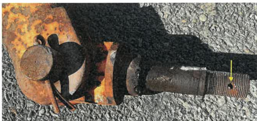
Figure 1 – Intact male threaded section on swivel (split pin passes through hole)
