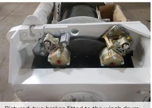
Pictured: two brakes fitted to the winch drum.
