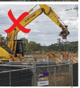
If any of these cannot be objectively proven, the excavator must not be used as a crane!
